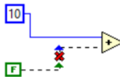
Figure 5.19 A example of wrong connection
